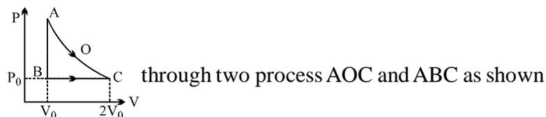
in the figure. Process AOC is isothermal
